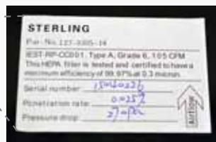
The HEPA filter is individually tested and certified to be 99.97% efficient at .3 microns according to IEST-RP-CC001 test requirement.
