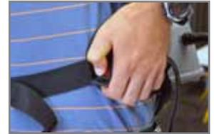
On-Off Switch: Hip mounted for easy access.
