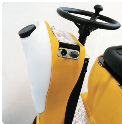
The detergent tank of the 3SD system.
