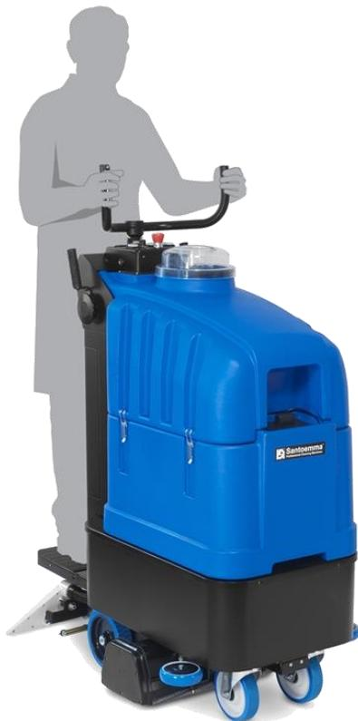
**Nikita** is a “step-on” carpet cleaning machine. It is ideal for very large areas of carpet and it is able to clean up to **1000 square metres** of carpet in 1 hour. In a single pass, a 70cm strip of carpet is sprayed with a concentrated chemical solution, brushed with two counter-rotating brushes, rinsed and vacuumed.
